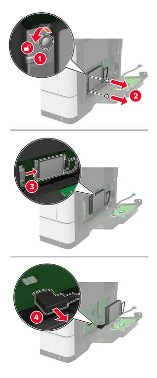
${\bm b}\$  Connect the ISP extended cable to the ISP connector.
