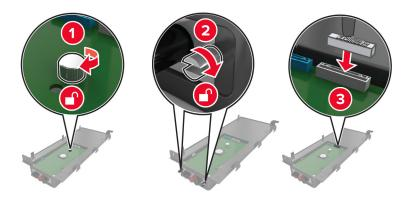
6 Open, and then remove the controller board access cover.
