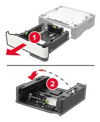
**5** Remove the used pick roller assembly.
