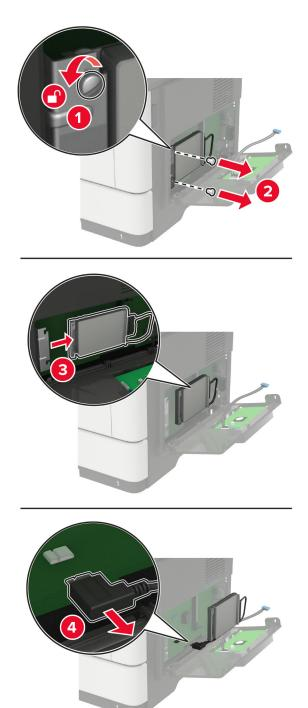
**b** Connect the ISP extended cable to the ISP connector.
