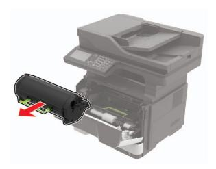
**3** Remove the used imaging unit.
