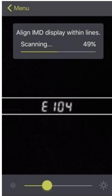
To scan the PDU, position the smart device so that the characters on the LED display are between the lines on the screen.
