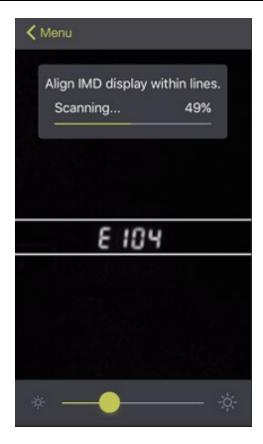
To scan the PDU, position the smart device so that the characters on the LED display are between the lines on the screen.
