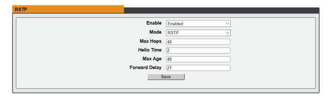
Use the RSTP section to Enable/Disable the RSTP Protocol, as well as make changes to RSTP settings.
