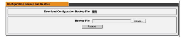
The Configuration Backup and Restore section allows the user to backup the PDU configuration file for future use in the case that the device is reset to defaults for any reason.
