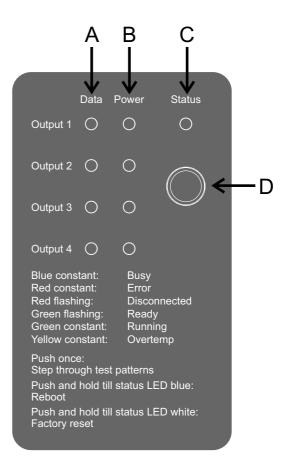
Figure 10: Status LEDs and control button
