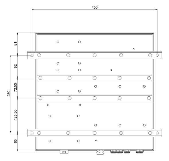
Figure 4: Mounting hole spacing (in mm)
