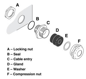
Figure 6: Cable gland assembly
