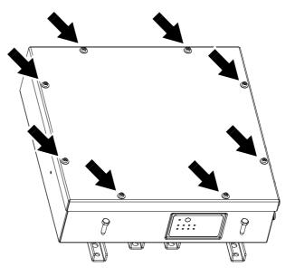
Figure 7: Cover retaining screws
