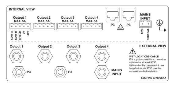
Figure 5: Power and data connections, internal and external views
