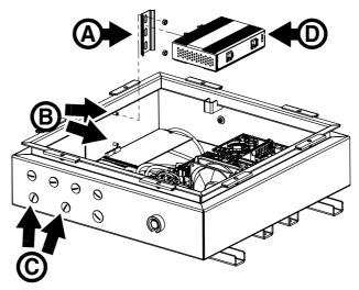
Figure 8: Installing a fiber-to-Ethernet converter
