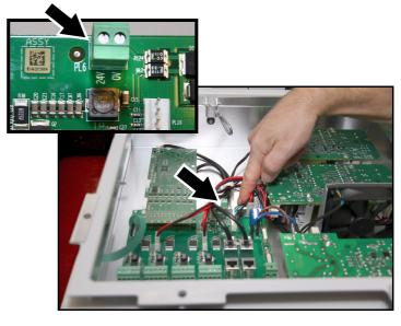
Figure 9: 24 VDC source at PL6
