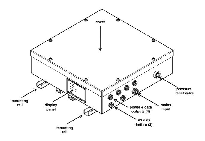
Figure 1: Parts identification
