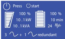
7. The UPS is now ready to operate, and displays the normal On/Off function screen. Press the ON button on the display screen to start the UPS.
