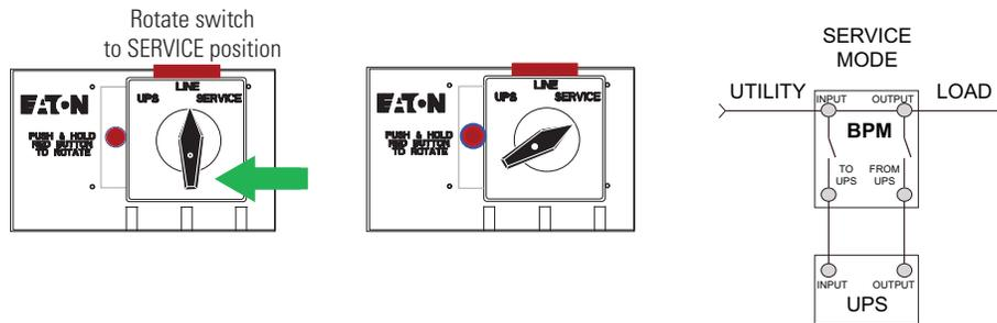
**Figure 23. Bypass From LINE to SERVICE**
