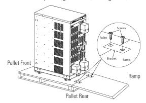
Figure 8. Moving the UPS from the Pallet
