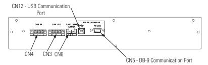
Figure 64. EBM Communication Ports
