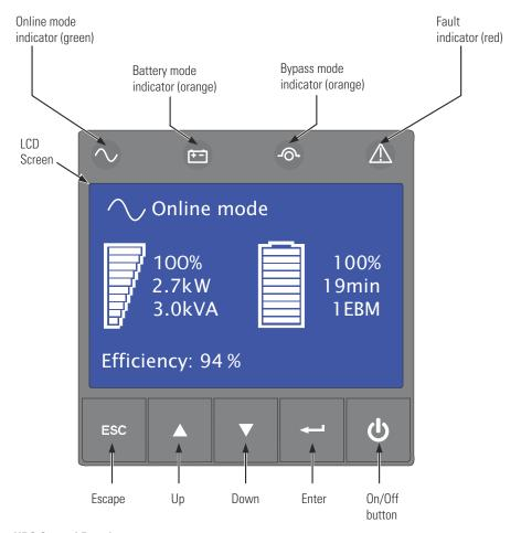
Figure 44. UPS Control Panel
