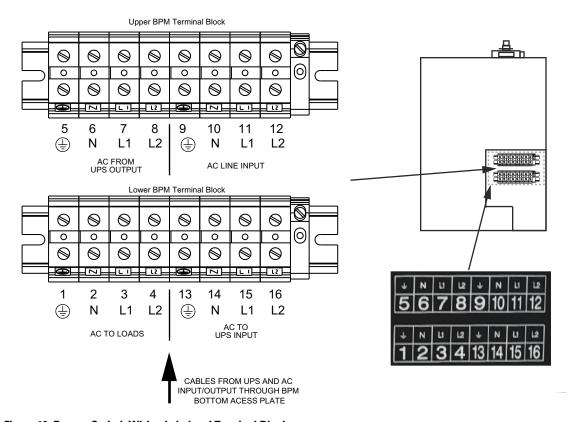
Figure 18. Bypass Switch Wiring Label and Terminal Blocks
