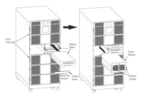
Figure 41. Inserting the Modules
