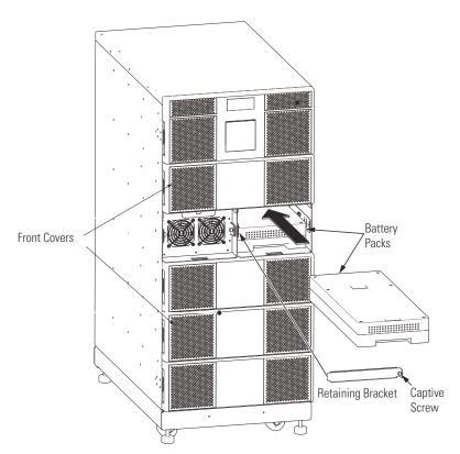
Figure 65. Battery Replacement
