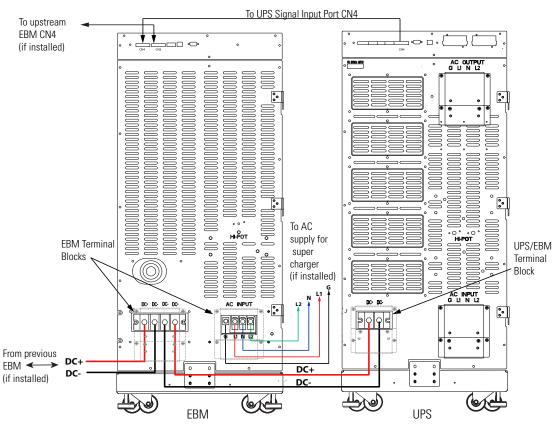
Figure 37. EBM to UPS Connections
