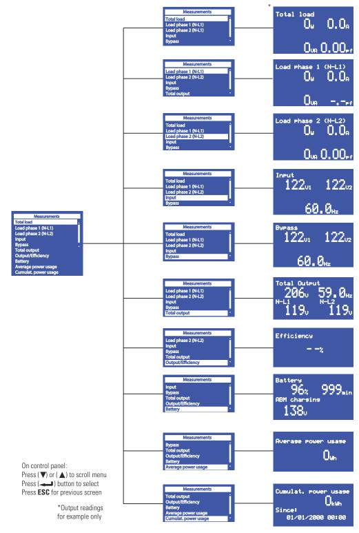
Figure 50. Measurements Menu
