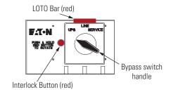
Figure 21. Bypass Switch Positions
