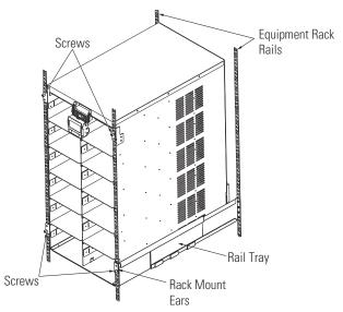
Figure 13. Securing the UPS in the Rack
