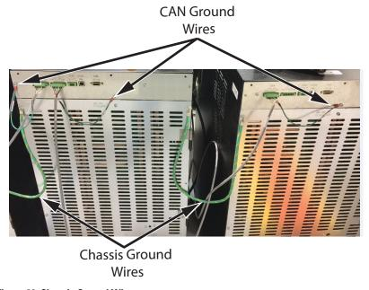
Figure 39. Chassis Ground Wires
