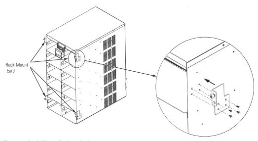
Figure 10. Rack-Mount Ear Installed
