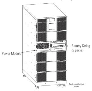
Figure 3. Power Modules and Battery Strings
