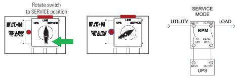
Figure 23. Bypass From LINE to SERVICE
