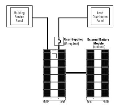
Figure 27. Typical Installation without a Bypass Switch
