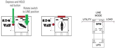
Figure 22. Bypass From UPS to LINE
