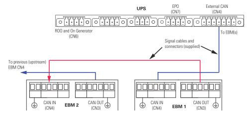
Figure 38. UPS Input Control Signal Wiring (for External Controls)
