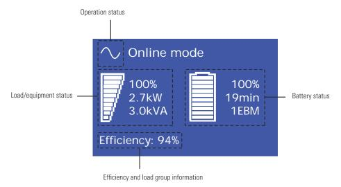
Figure 45. LCD Display Status Indicators
