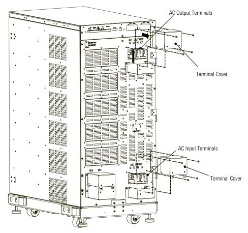
Figure 15. UPS AC Power Terminal Access
