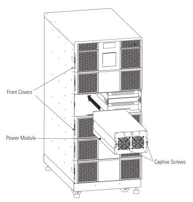
Figure 66. Power Module Replacement
