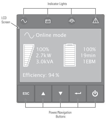
Figure 6. UPS Control Panel
