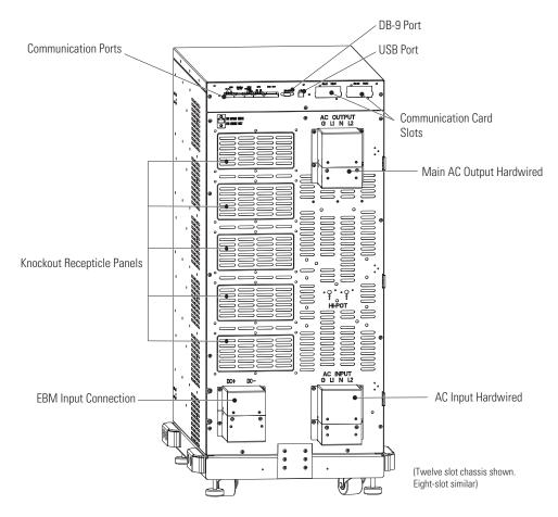
Figure 2. Twelve-Slot Rear View Access
