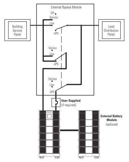
Figure 14. Typical Installation with a Bypass Switch
