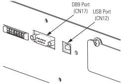
**Figure 43. Communication Ports**
