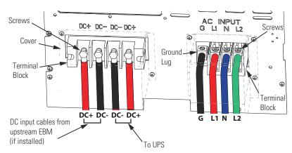
Figure 33. Battery Cable Assembly Installation.
