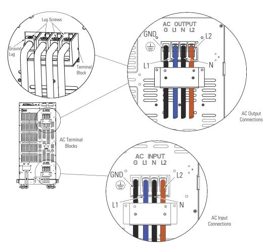
Figure 30. UPS Input and Output Terminal Connections
