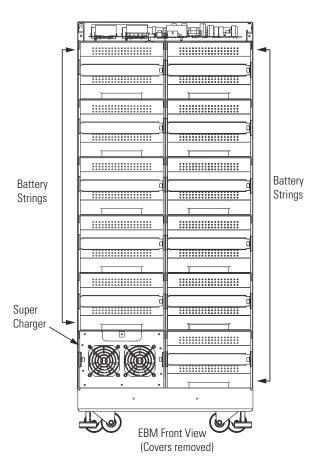
Figure 42. EBM Battery Strings and Charger
