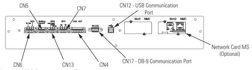
Figure 63. UPS Communication Ports
