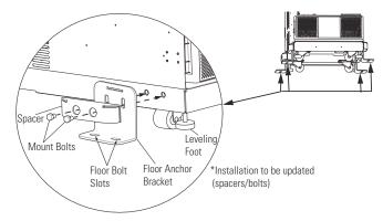
**Figure 9. Floor Anchor Bracket Installation**
