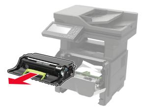
**Warning—Potential Damage:** Do not expose the imaging unit to direct light for more than 10 minutes. Extended exposure to light may cause print quality problems.
