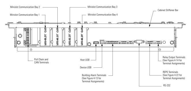
Figure 4-10. Interface Terminal Detail
