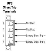
Figure 4-17. Battery Shunt Trip Terminal Assignments
