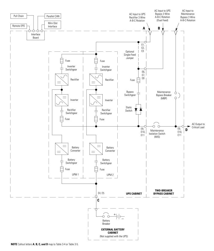
Figure 5-11. Eaton 93PM-100-2 UPS System with Two-Breaker Bypass Oneline
