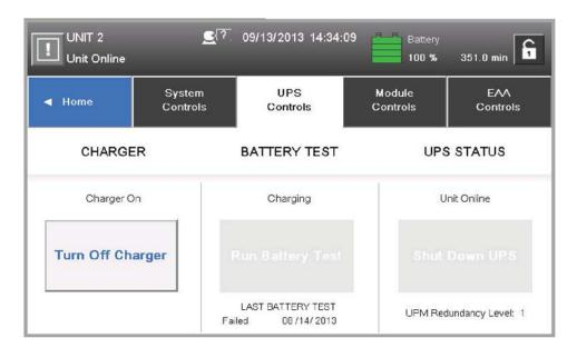
Figure 6-17. Typical UPS Control Screen
