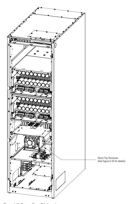
Figure 4-15. Battery Shunt Trip Location
