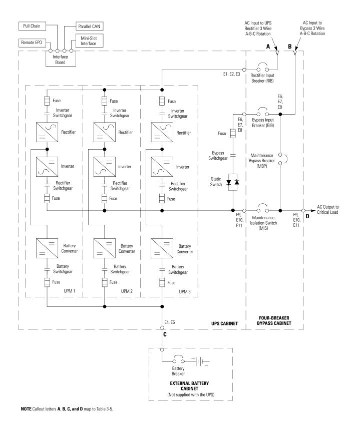
Figure 5-17. Eaton 93PM-100-3 UPS System with Four-Breaker Bypass Oneline
