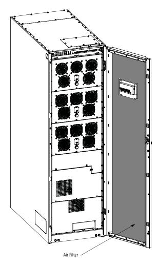
Figure 8-1. Air Filter Location
