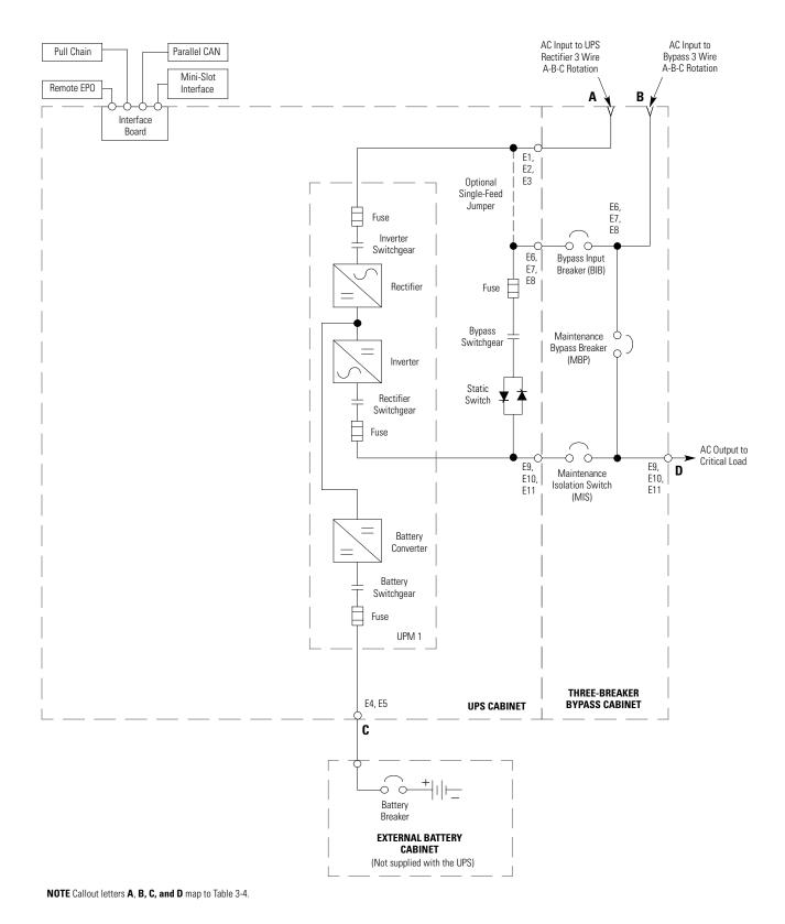
Figure 5-8. Eaton 93PM-100-1 UPS System with Three-Breaker Bypass Oneline
