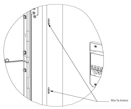
Figure 4-12. Wire Tie Anchors
