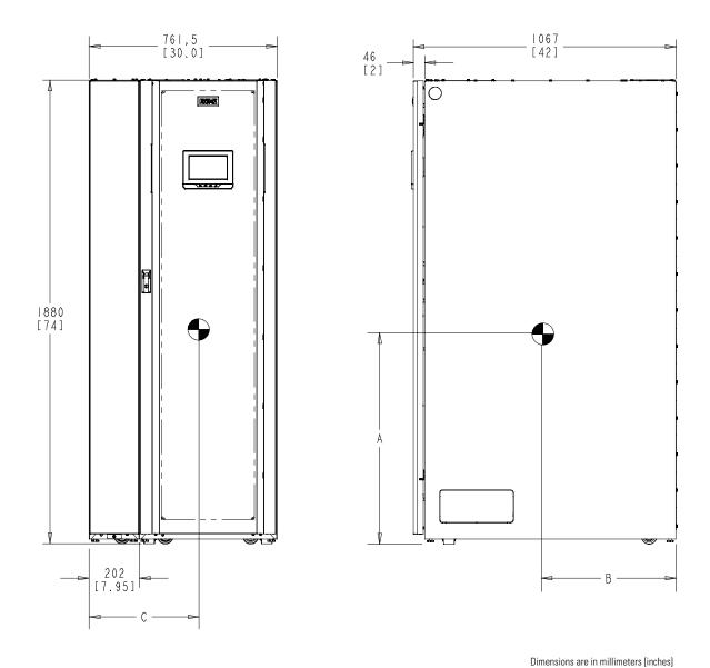
Figure 3-7. UPS Cabinet with Left-Mounted or Right-Mounted Sidecar Center of Gravity
