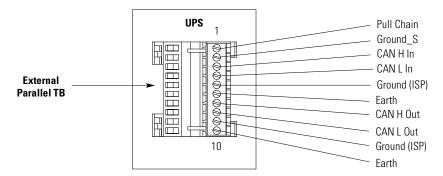
Figure 4-19. External Parallel Terminal Block
