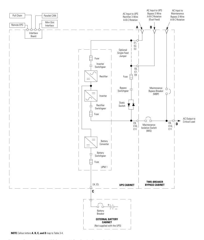
Figure 5-7. Eaton 93PM-100-1 UPS System with Two-Breaker Bypass Oneline
