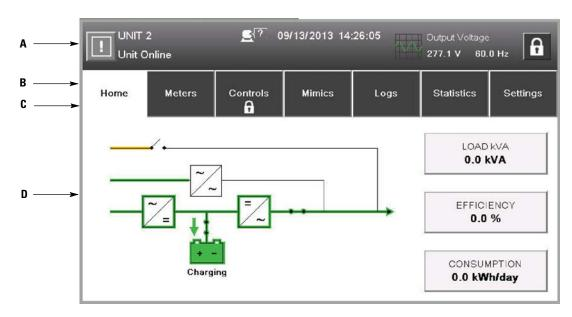
Figure 6-3. Parts of the LCD
