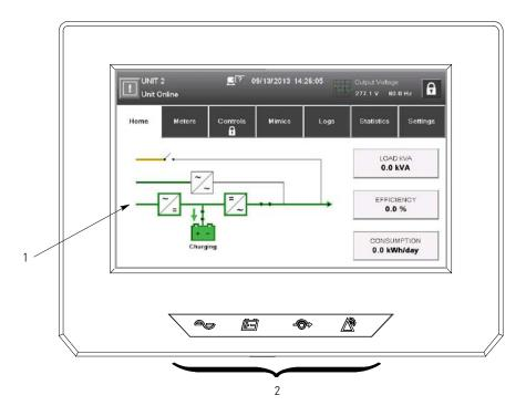
Figure 6-2. UPS Control Panel
