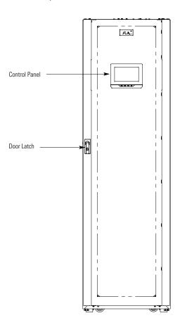
Figure 6-1. UPS Controls and Indicators
