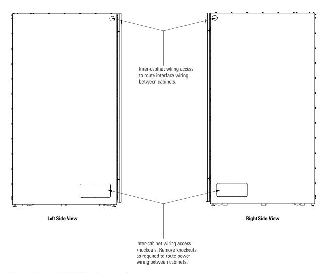
Figure 4-6. UPS Inter-Cabinet Wiring Access Location
