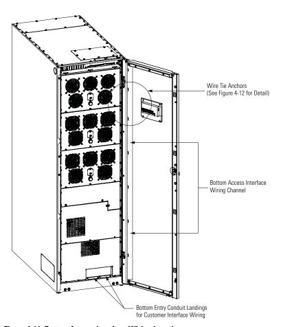
Figure 4-11. Bottom Access Interface Wiring Location
