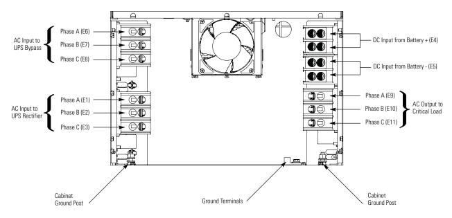
Figure 4-8. Power Terminal Detail
