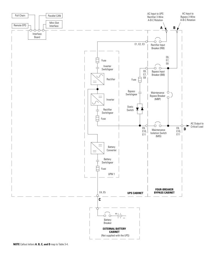
Figure 5-9. Eaton 93PM-100-1 UPS System with Four-Breaker Bypass Oneline
