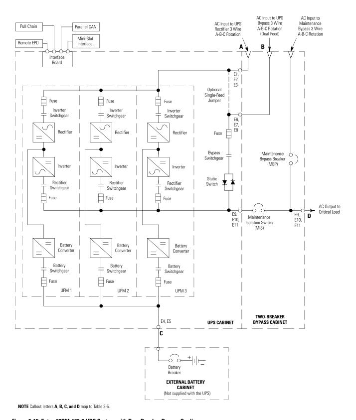
Figure 5-15. Eaton 93PM-100-3 UPS System with Two-Breaker Bypass Oneline
