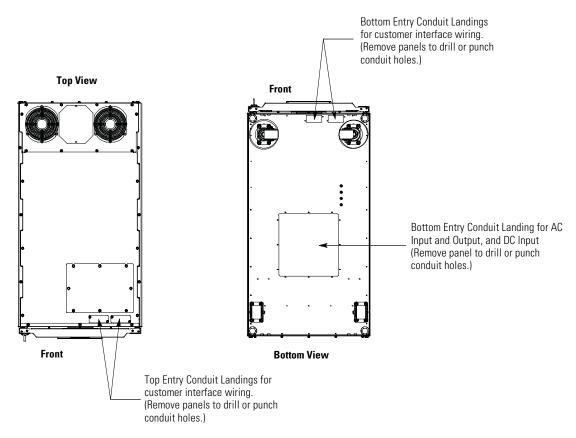
Figure 4-4. UPS Conduit and Wire Entry Locations
