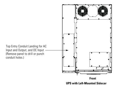
Top Entry Conduit Landing for AC Input and Output, and DC Input (Remove panel to drill or punch conduit holes.)
