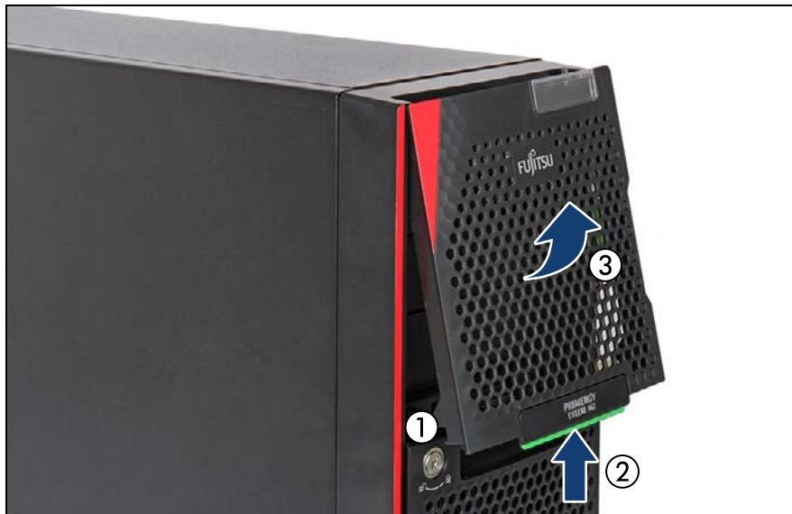
Figure 21: Removing the accessible drive bay cover
