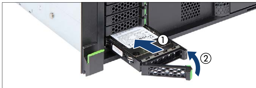
Figure 26: Installing the 2.5-inch HDD/SSD module
