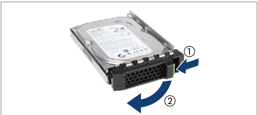
Figure 28: Opening the 3.5-inch HDD module locking lever
