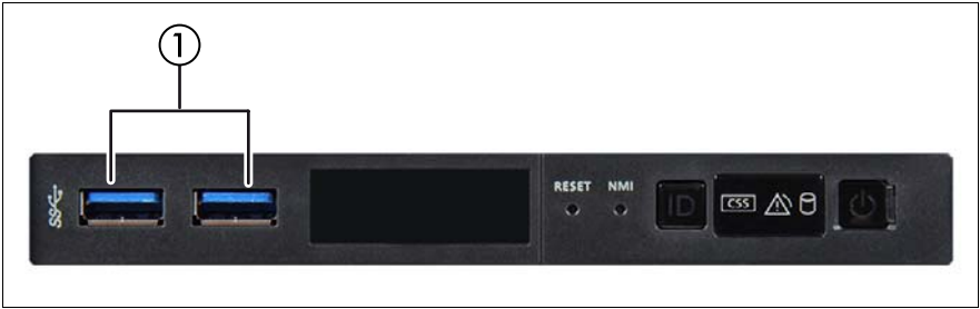
Figure 5: Connectors on the front panel
