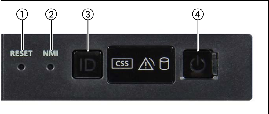
Figure 7: Controls on the front panel module
