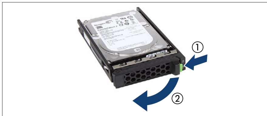
Figure 25: Opening the 2.5-inch HDD/SSD module locking lever
