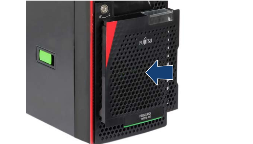
Figure 22: Placing the accessible drive bay cover
