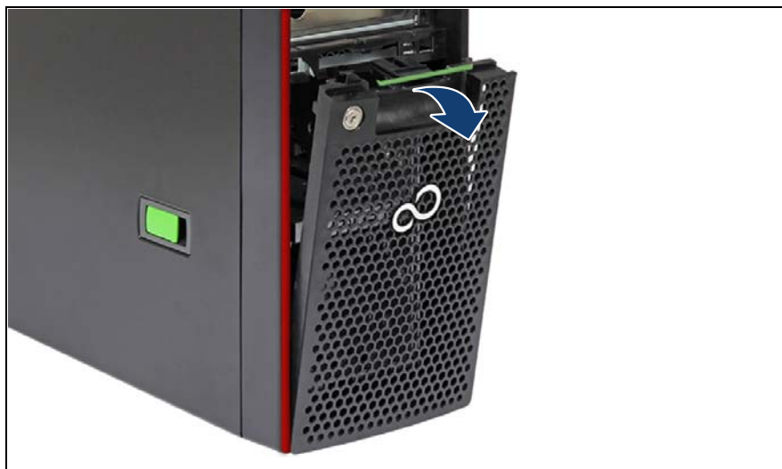
Figure 23: Removing the HDD bay cover
