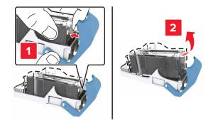
**4** Insert the new cartridge into the cartridge holder.
