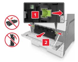
**3** Unlock the photoconductor unit.
