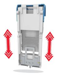
7 Push the cartridge holder into the finisher until the holder *clicks* into place.
