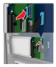
To install a hard disk directly on the controller board cage:
