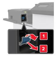
**3** Remove the empty staple cartridge from the cartridge holder.
