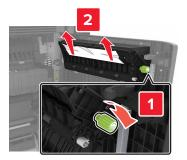
**4** Open the standard trays, and then locate the jammed paper.
