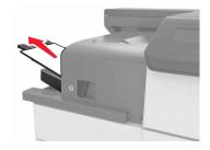
2 Press the latch on the staple finisher, and then slide the finisher to the left.
