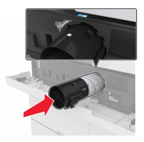
**5** Rotate the cartridge clockwise to lock it into place.
