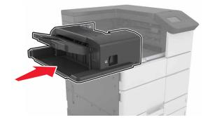
**4** Open door C, and then remove the jammed paper.
