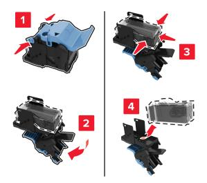
**4** Insert the new cartridge into the cartridge holder.
