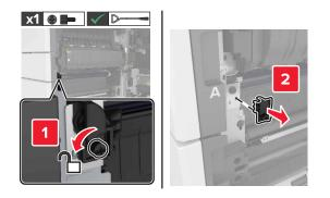
**4** Loosen the screws of the transfer module lock.
