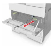
**5** Remove the printhead wiper.
