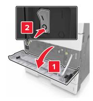
2 Open door C. Make sure that it does not hit any cable attached to the printer.
