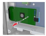
**6** Secure the ISP mounting bracket to the controller board cage using the screws.
