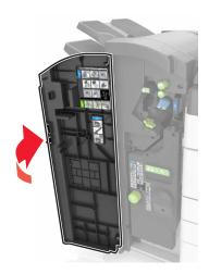
4 Remove the jammed paper from any of the following locations:Note: Make sure that all paper fragments are removed.
