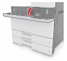
7 Clean the charger and the printhead lens. For more information, see <u>"Cleaning the charger and the printhead lens"</u> on page 129.
