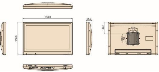
Figure 1.1 Dimensions of the POC-W213L Series
