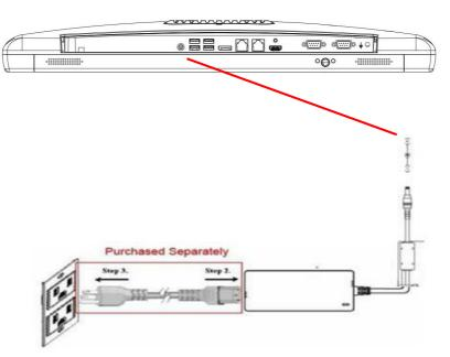
Figure 2.4 Connecting the power cord
