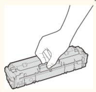
To avoid scratching the surface ( [a]) of the drum inside the machine or exposing it to light. Do not touch the electrical contacts ( ) or the toner cartridge memory ( ).
