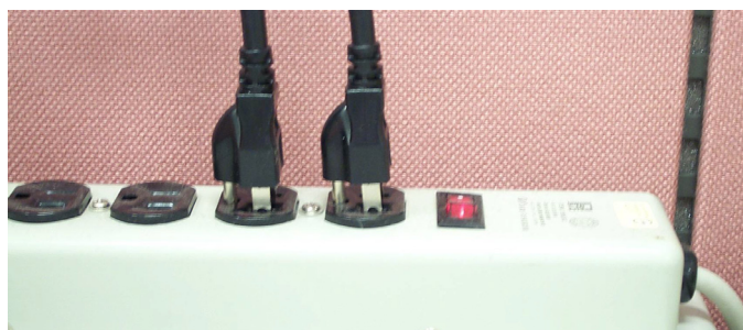
Figure 3.5: Power cord plugs should have same orientation in the socket/ 插座上电源线方向相同 / 插座上的電源線方向應相同
