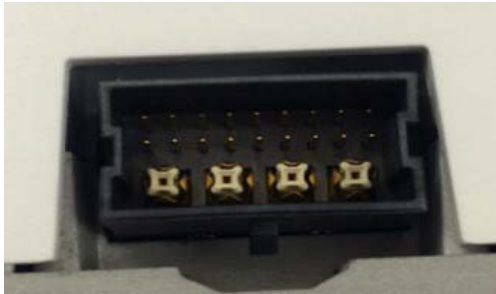
Figure 11 Smart Antenna Connector C9120AXE and C9120AXP Models
