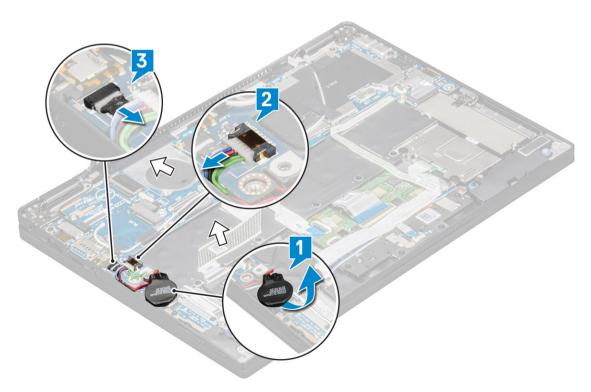
6 Peel the tapes that secure antenna cables and remove the cables from the routing clips.
