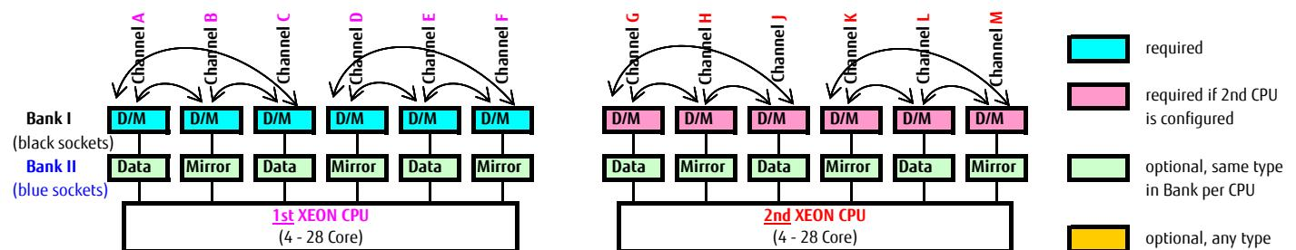
Mirrored Channel Mode requires identical modules on channel A, B, C, D, E, F (1st CPU) or channel G, H, J, K, L and M (2nd CPU) 50% of the capacity is used for the mirror => the available memory for applications is only half of the installed memory. If this mode is used, a multiple of 6 identical modules has to be ordered.
