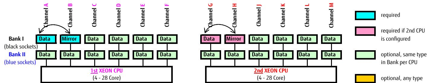
Mirrored Channel Mode (2 DIMMs per CPU) requires identical modules on channel A & B (1st CPU) or channel G & H (2nd CPU) 50% of the capacity is used for the mirror => the available memory for applications is only half of the installed memory. If this mode is used, a multiple of 2 identical modules has to be ordered.
