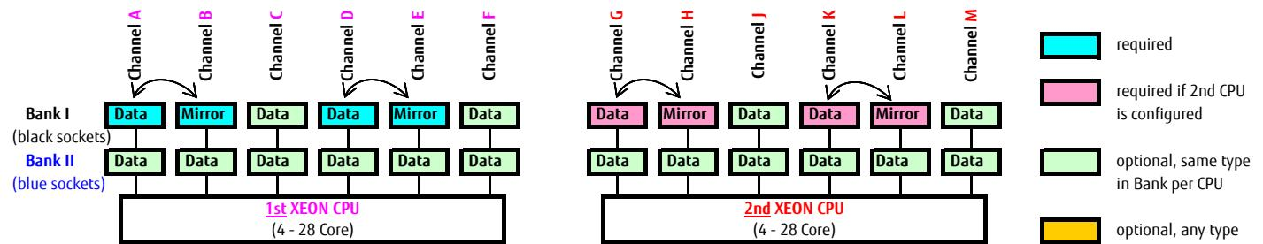
Mirrored Channel Mode (4 DIMMs per CPU) requires identical modules on channel A, B, D & E (1st CPU) or channel G, H, K & L (2nd CPU) 50% of the capacity is used for the mirror => the available memory for applications is only half of the installed memory. If this mode is used, a multiple of 4 identical modules has to be ordered.
