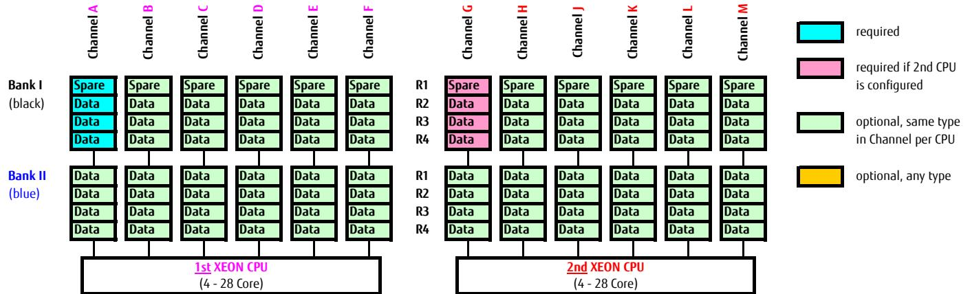
Rank Sparing Mode requires identical modules (same capacity and technology) within the same channel. The available memory for applications will vary depending on configuration. Please refer to the spreadsheet above "Effective Memory capacity with active Rank Spared Mode". Population rule for Rank sparing mode is to achieve max. available memory, e.g. 4 DIMMs will be spread across two channels, each with 2DPC
