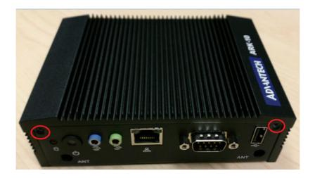
Remove aluminum top chassis and install RAM.
