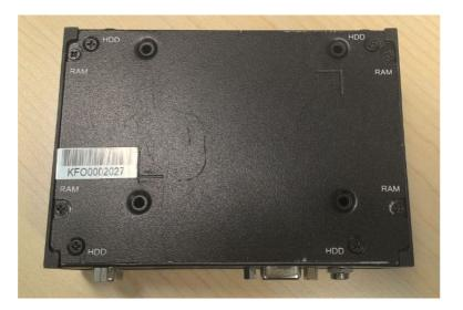
2. Unscrew the four screws on the sides of ARK-10.
