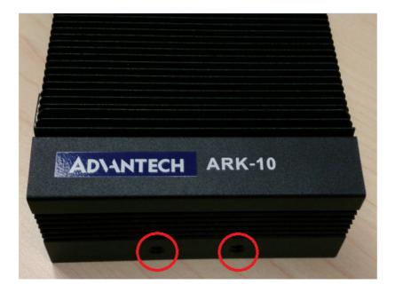
3. Unscrew the four screws on the front/rear face plate of ARK-10.
