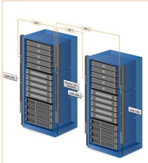
Multi-Linking View in the Equipment Cabinet
