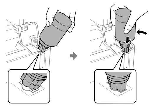
5. Wait for the ink to fill the tank. Ink flows into the tank and stops automatically when the ink is filled to the upper line.
