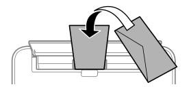
Load one sheet of loose-leaf or other paper with holes facing as shown. You can load one sheet at a time in only these sizes: Letter (8.5 × 11 inches [216 × 279 mm]), A4 (8.3 × 11.7 inches [210 × 297 mm]), or Legal (8.5 × 14 inches [216 × 356 mm]).
