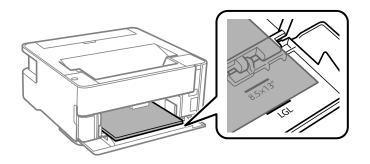
• For 8.5 × 13 inch (216 × 330 mm) paper, load paper using the guide line as shown.
