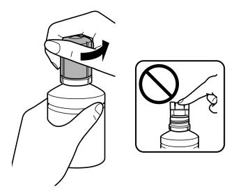
**Caution:** Do not shake or squeeze the bottle. Do not touch the top of the bottle after its cap is removed.
