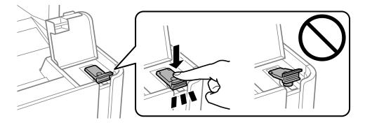
**Note:** If any ink remains in the bottle, replace the bottle cap and tighten it. Store the bottle upright for later use.
