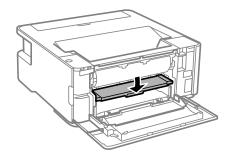
4. Remove any jammed paper from the front of the printer.
