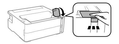
8. If the ◊ ink light is flashing, press the ♥ stop button.
