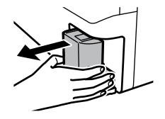
Note: Do not tilt the used maintenance box until after it is sealed in the plastic bag or ink may leak.
