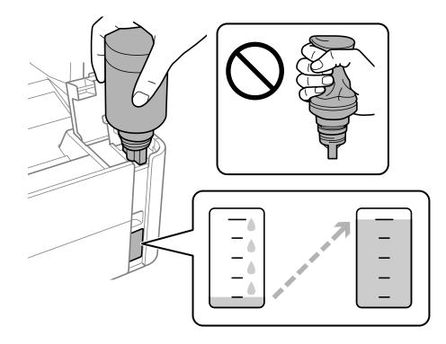
Note: If ink does not flow from the bottle, lift and reinsert the bottle.
