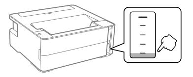
**Caution:** If the ink level is below the lower line on the ink tank, fill it to the upper line on the ink tank. Continued use of the product when the ink level is below the lower line on a tank could damage the product.
