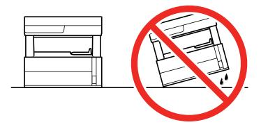
• Do not lift the product by gripping the scanner unit. Make sure you lift using the handholds on the bottom of the product.
