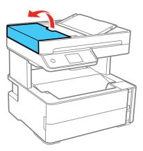
6. Use a soft, moist, lint-free cloth (microfiber is recommended) to clean the rollers and the interior of the ADF.
