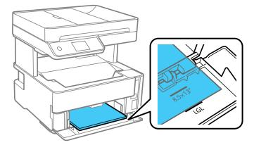
• For  $8.5 \times 13$  inches (216  $\times$  330 mm) paper, load paper using the guide line as shown.
