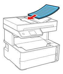
**Note:** Do not load originals above the arrow mark on the ADF edge guide.
