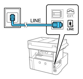
**Note:** If you have a DSL or ISDN connection, you must connect the appropriate DSL filter, or ISDN terminal adapter or router to the wall jack to be able to use the line for faxing or voice calls using your product. Contact your DSL or ISDN provider for the necessary equipment.
