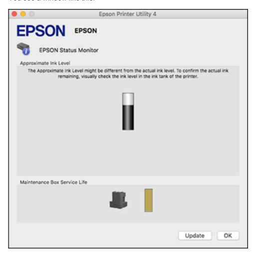
3. Refill the ink tank or replace the maintenance box as needed.
