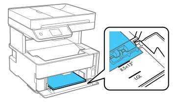
• Insert up to 10 envelopes with the printable side facedown and flap edge left, as shown.
