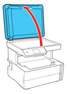
2. Place your original facedown on the scanner glass with the top facing into the corner. Slide the original to the edges of the indicated corner.
