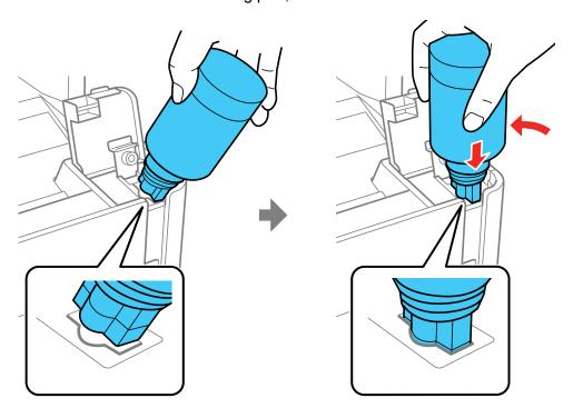
8. Wait for the ink to fill the tank. Do not squeeze the bottle. Ink flows into the tank and stops automatically when the ink is filled to the upper line.
