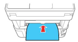
• Load one envelope in the center of the rear paper feed slot. Load it printable side up and flap edge left.
