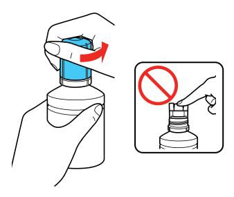
**Caution:** Do not shake or squeeze the bottle. Do not touch the top of the bottle after its cap is removed.
