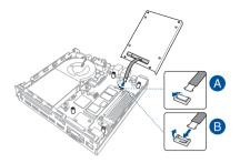
5. Replace the storage bay and secure it with the four (4) screws removed previously.
