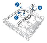
3. Align and insert the memory module into the slot (A) and press it down (B) until it is securely seated in place.
