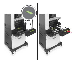
**Warning—Potential Damage:** When replacing a toner cartridge, do not leave the imaging unit exposed to direct light for an extended period of time. Extended exposure to light may cause print quality problems.
