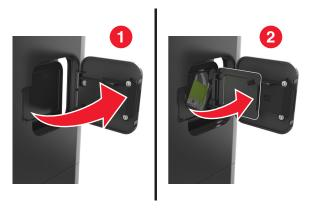
**2** Pull down the latch of the staple cartridge holder, and then pull the holder out of the finisher.
