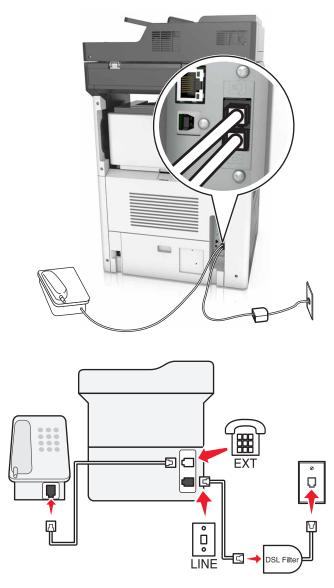
Digital subscriber line (DSL) splits your regular telephone line into two channels: voice and Internet. Telephone and fax signals travel through the voice channel, and internet signals pass through the other channel.
