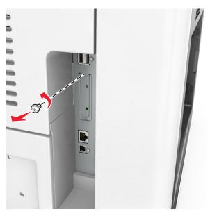
**b** Lift the metal cover, and then pull it out completely.
