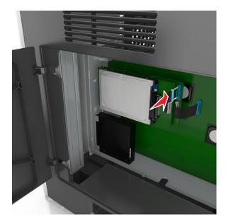
To install a printer hard disk directly on the controller board cage:
