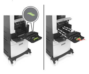
**7** Insert the toner cartridge into the printer by aligning the side rails of the cartridge with the arrows on the side rails inside the printer.
