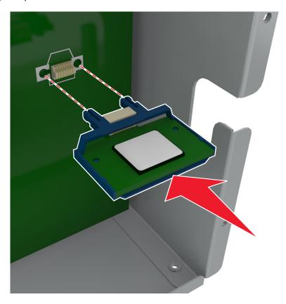
**Warning—Potential Damage:** Improper installation of the card may cause damage to the card and the controller board.
