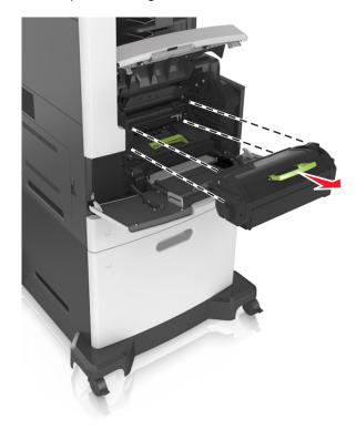
Lift the green handle, and then pull out the imaging unit from the printer.
