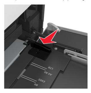
**Note:** Use the paper size indicators on the bottom of tray to help position the guides.
