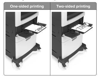
**Note:** If the holes on the long edge of the paper are on the left side of the tray, then a jam may occur.
