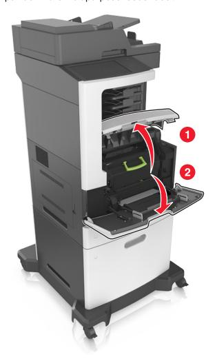
**2** Pull the cartridge out of the printer using the handle.
