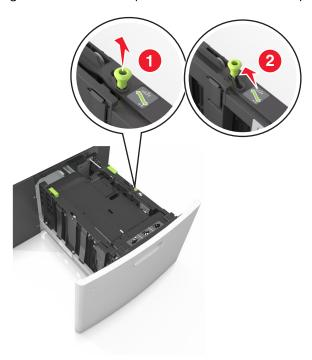
**b** If the A5 length guide is still attached to the length guide, then remove it from its place. If the A5 length guide is not attached, then proceed to step d.
