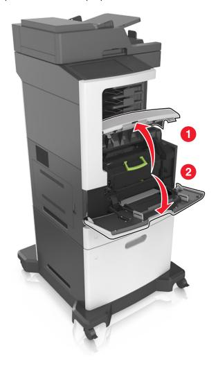
Pull out the toner cartridge from the printer using the handle.
