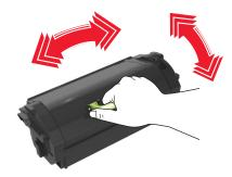
**4** Insert the toner cartridge into the printer by aligning the side rails of the cartridge with the arrows on the side rails inside the printer.
