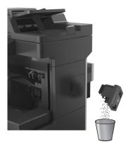
**3** Insert the emptied hole punch box back into the finisher until it *clicks* into place.
