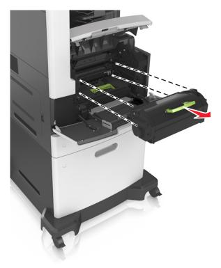
**3** Unpack the new toner cartridge, then remove the packing material, and then shake the cartridge to redistribute the toner.
