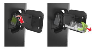
Open the staple guard, and then remove the loose staples.
