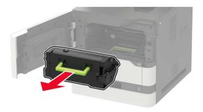
**3** Remove the used imaging unit.
