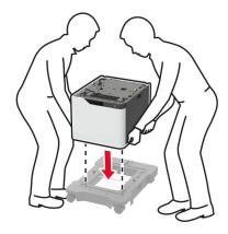
**5** Align the printer with the tray, and then lower the printer until it *clicks* into place.
