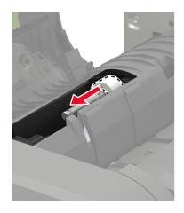
**6** Unpack the new ADF torque limiter.
