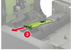
**4** Remove the used ADF separator roller.
