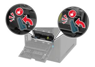
**3** Remove the used fuser.
