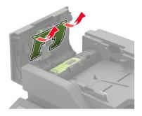
4 Remove the used ADF pick roller.
