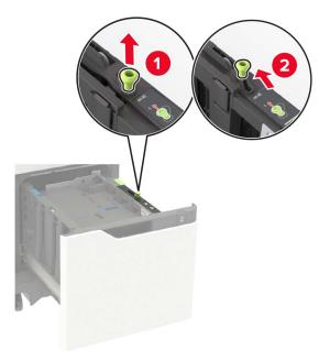
**b** If the A5 length guide is still attached, then remove it. If the guide is not attached, then proceed to <u>step</u> <u>d on page 33</u>.
