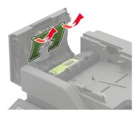
**4** Remove the used ADF feed roller.
