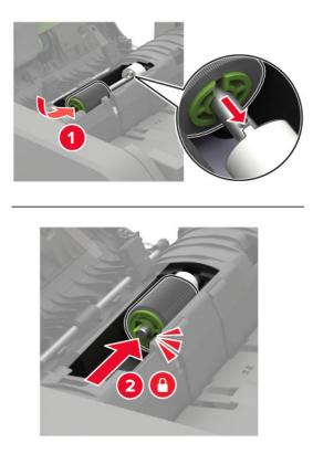
7 Insert the ADF separator roller cover until it *clicks* into place.
