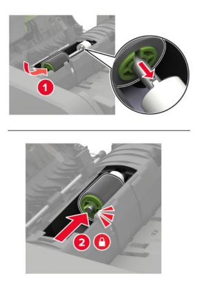
**9** Insert the ADF separator roller cover until it *clicks* into place.
