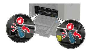
**4** Remove the used hot roll fuser.
