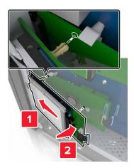
**8** Insert the plug of the hard disk interface cable into the connector on the ISP, and then connect the ISP solution interface cable into the receptacle of the controller board.
