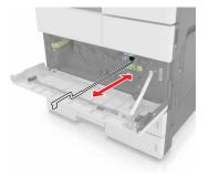
Remove the printhead wiper.
