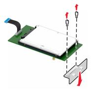
**7** Align the standoffs of the hard disk with the holes on the ISP, and then press the hard disk down until the standoffs *click* into place.
