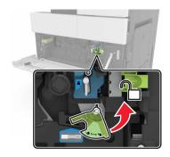
**4** Remove the photoconductor unit.
