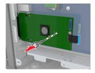
**5** Secure the ISP mounting bracket to the controller board cage using the screws.
