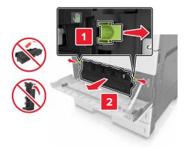
**3** Unlock the photoconductor unit.
