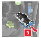
**3** Remove the empty staple cartridge from the cartridge holder.
