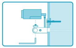
**2.** Fasten the camera to the ADA Camera Mount with the hex key.
