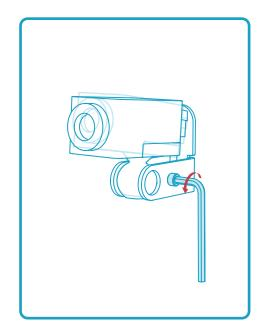
Loosen the screw with the hex hey to adjust camera orientation, and then tighten it.
