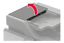
**3** Remove the ADF separator roller cover.
