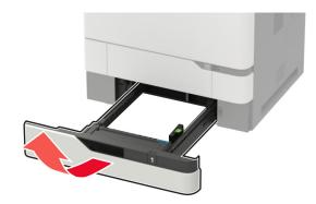
**Warning—Potential Damage:** A sensor inside the optional tray is easily damaged by static electricity. Touch a metal surface before removing the jammed paper in the tray.
