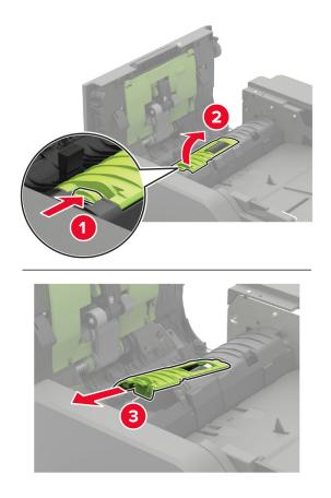
**4** Remove the ADF separator roller.
