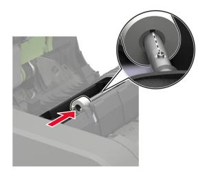
**8** Insert the ADF separator roller until it *clicks* into place.
