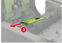
**4** Remove the used ADF separator roller.
