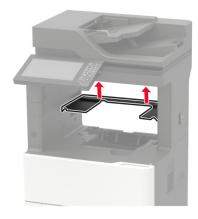
**5** Install the staple finisher to the printer, and then push it down to make sure that it is securely attached to the printer.
