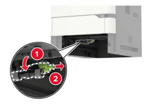
4 Using a damp, soft, lint-free cloth, wipe the pick tires.Note: Apply isopropyl alcohol to the cloth.
