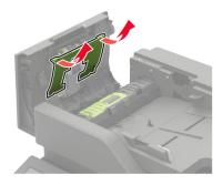
4 Remove the used ADF pick roller.
