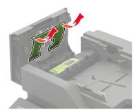
**4** Remove the used ADF feed roller.
