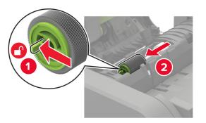
**5** Remove the used ADF torque limiter.
