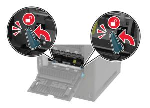
Remove the used fuser.
