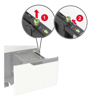
**b** If the A5 length guide is still attached, then remove it. If the guide is not attached, then proceed to <u>step</u> <u>d on page 32</u>.
