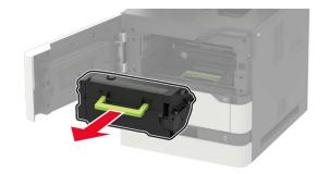
**3** Remove the used imaging unit.
