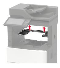
5 Install the finisher to the printer, and then push it down to make sure that it is securely attached to the printer.
