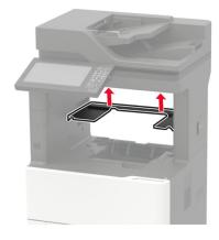
**5** Install the offset stacker to the printer, and then push it down to make sure that it is securely attached to the printer.
