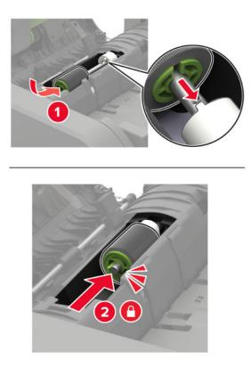
7 Insert the ADF separator roller cover until it *clicks* into place.
