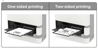
• Load envelopes with the flap side down and against the left side of the paper guide.
