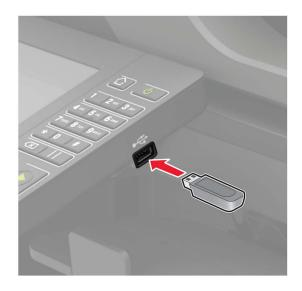
**3** Touch **Scan to USB** and adjust the settings if necessary.
