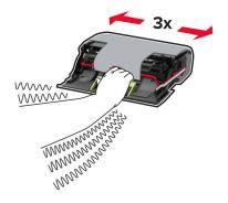
**Warning—Potential Damage:** Do not expose the imaging unit to direct light for more than 10 minutes. Extended exposure to light may cause print quality problems.
