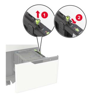
**b** Squeeze and slide the length guide to the position for A5 until it *clicks* into place.
