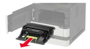
**4** Remove the used transfer roller.
