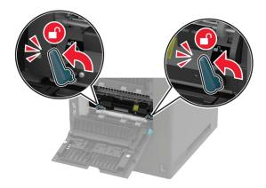
**3** Remove the used fuser.
