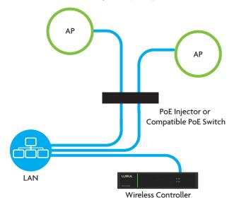
Access Point Placement: Place APs to ensure adequate coverage, but not so far apart that there is no signal overlap. You may have to experiment with AP placement to optimize the roaming experience. The APs should overlap enough that the client device has a good connection to the AP to which it is currently attached, but also sees the next-nearest AP.
