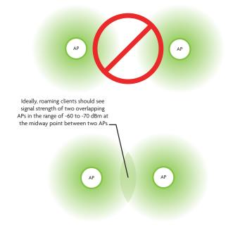
Note: Visit <u>luxul.com/ap-placement</u> for details on how to select and optimize AP placement. ✓ Note: Consider using Ekahau HeatMapper to assist with this process, available from <u>www.ekahau.com</u>. Luxul also offers an informative "How-To" video on HeatMapper at <u>luxul.com/</u> <u>how-to-videos</u>.
