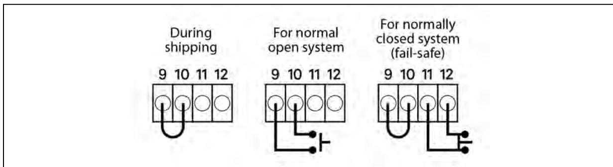
**NOTE:** A jumper is factory-installed between Pins 9 and 10 to disable the Main Control Switch, which prevents the UPS from being started accidentally during shipment and installation. This jumper must be removed before the unit can be started. If the installation does not require connection to a REPO system, the factory-installed jumper must be removed.
