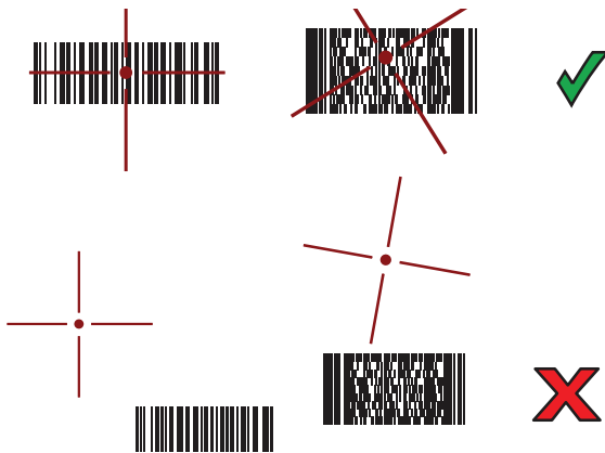
Figure 26 RS507/RS507X Aiming Pattern
