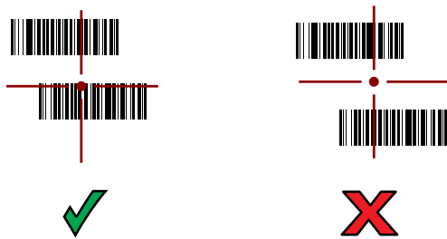
Figure 29 RS5100 Pick List Mode with Multiple Barcodes in Aiming Pattern
