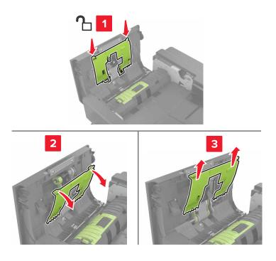
**4** Remove the ADF feed roller.
