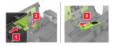
**4** Remove the ADF separator roller.
