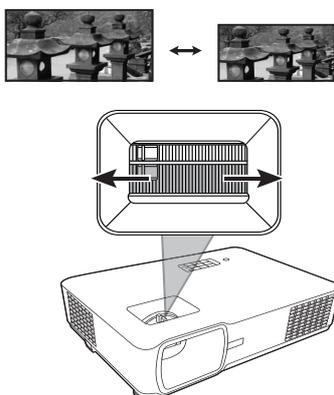
To improve the clarity of the image, rotate the Focus Ring.
