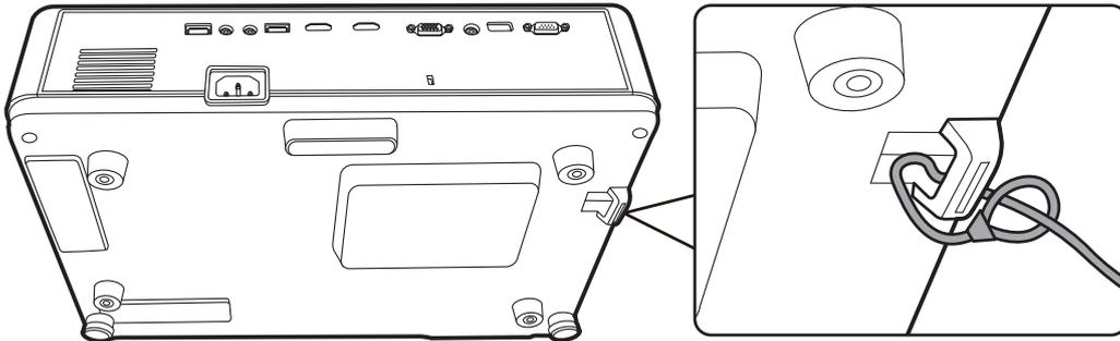
**NOTE:** The security slot can also be used as a safety anchor if the projector is mounted to the ceiling.
