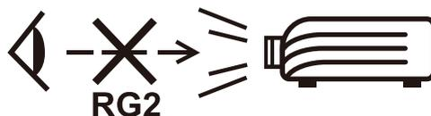
**CAUTION:** Possibly hazardous optical radiation is emitted from this product. As with any bright light source, do not stare into the beam,
