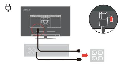
9. Connect the cables with cable clip.
