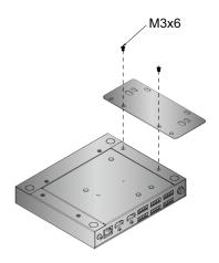
2. Screw the bracket into any convenient location on the rack.
