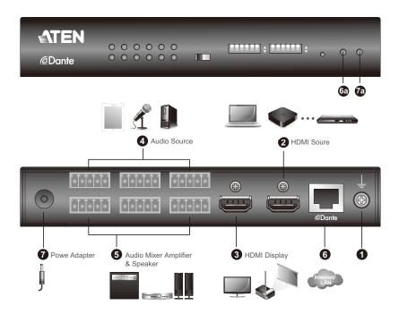
1. Ground the VE66DTH by connecting one end of a grounding wire to the ground terminal and the other end to a suitable grounded object.
