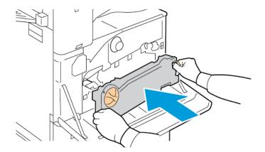
b. Press the waste toner transport unit toward the printer, until both ends click into place.
