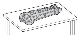
Caution: To avoid toner spills, do not lay the waste toner transport unit face down, or on its side.
