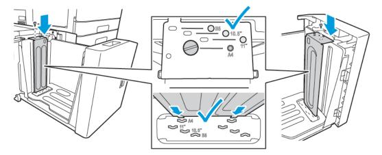
4. On the top of the side gate, lift the pin, then guide it into the required paper size in the slot. To lock the side gate into place, release the pin.
