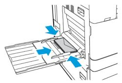
• For envelopes with a self-seal flap on a short edge, load envelopes face down with the flaps closed, and flaps toward the right.
