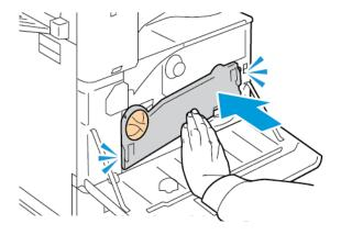
c. To lock the waste toner transport unit, rotate the locking lever 45 degrees clockwise.
