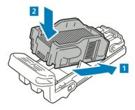
7. Grasp the new staple cartridge by the orange handle, then insert the cartridge into the stapler assembly until it clicks.
