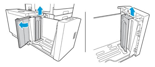
3. For the rear spacer plate, place the tabs at the bottom of the plate into the slots that correspond with the correct paper size. Slide down the spacer plate, then engage the peg on the top of the tray with the matching hole in the spacer plate. To secure the spacer plate, install the screw. Repeat the procedure for the spacer plate at the front of the tray.
