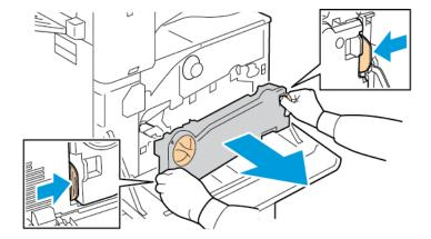
c. Place the removed waste toner transport unit on a level surface, with the openings facing up.
