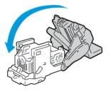
8. To return the staple cartridge to the booklet maker, insert the staple cartridge and push up on the cartridge handle as shown.
