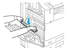
8. Remove the protective cover from the transfer roller, then close Door A.
