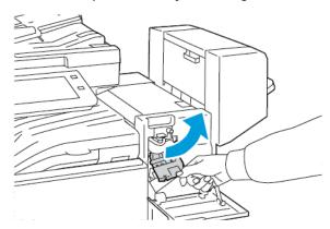
4. To remove the staple cartridge, grasp the orange handle, then pull the handle toward you.
