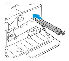
7. Push the belt cleaner until it clicks into place, then to lock the belt cleaner, turn the orange lever to the right.
