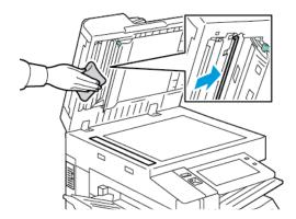
4. Return the document cover to the original position, and ensure that the lever is locked in place. If you touch the document cover, before you close the document feeder, clean the cover.
