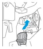
7. Return the stapler assembly to the original position, then close the finisher door.
