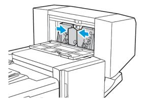
3. Hold the tabs on both sides of the staple cartridge and pull the cartridge out of the finisher.
