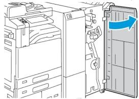
2. Grasp the stapler assembly lever R1, then move the lever to the right.
