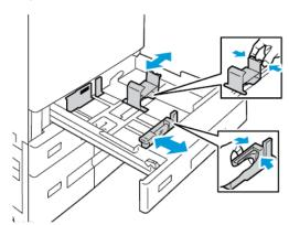
3. To move out the paper-length guide, pinch the guide lever and slide the guide outward.
