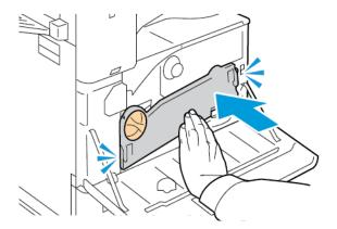
c. To lock the waste toner transport unit, rotate the locking lever 45 degrees clockwise.
