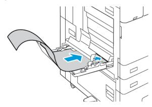
4. Carefully roll the remaining length of the banner paper into the Long Sheet Feed Extension guides. Ensure that the trailing edge rests against the front guide.
