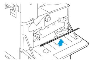
4. Slowly push the cleaning rod into the printhead LED lens cleaning slot until it stops, then pull out the rod. Repeat this action two more times.
