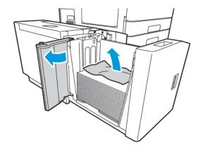
7. Reload the tray with undamaged paper, close the side gate, then close the tray.
