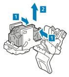
6. Insert the front side of the new staple pack into the staple cartridge, then push the rear side into the cartridge.
