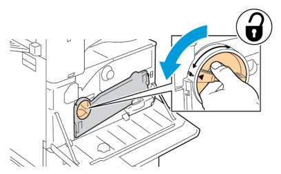
b. To release the waste toner transport unit, press both orange tabs as shown, then pull out the unit from the printer.
