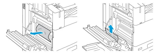
4. If paper is jammed on the inside of door A, lift handle A3, then remove the jammed paper. Return handle A3 to the original position.
