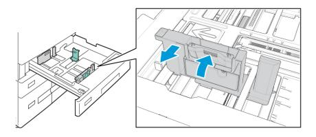
4. To move out the paper-width guide, pinch the guide lever and slide the guide outward.
