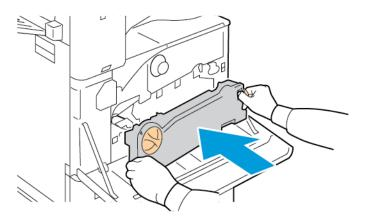
b. Press the waste toner transport unit toward the printer, until both ends click into place.
