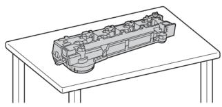
Caution: To avoid toner spills, do not lay the waste toner transport unit face down, or on its side.
