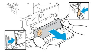
c. Place the removed waste toner transport unit on a level surface, with the openings facing up.
