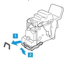
9. To return the staple cartridge to the booklet maker, insert the staple cartridge, then push up on the cartridge handle as shown.
