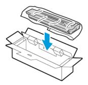
6. Hold the left side of the new waste container and slide it into the printer until it clicks.
