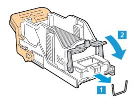
8. Grasp the orange handle, then insert the cartridge into the stapler assembly until the cartridge clicks into place.
