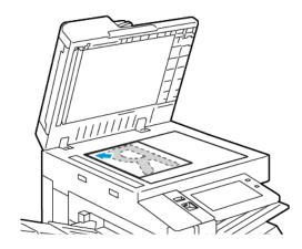
• For multiple, single, or 2-sided pages, use the duplex automatic document feeder. Remove any staples and paper clips from the pages. Insert the original documents face up in the duplex automatic document feeder, with the top of the page entering the feeder first. Adjust the paper guides so that they fit against the original documents.
