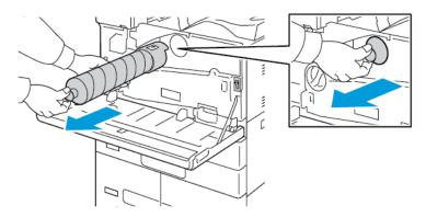
3. Remove the new toner cartridge from the packaging. Tilt the cartridge up and down, then left and right 10 times.
