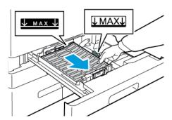
• For short-edge feed, insert labels face up with the top edge toward the right.
