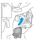
7. Return the stapler assembly to its original position, then close the finisher door.
