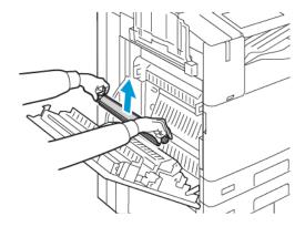
6. Place the used transfer roller in the plastic bag.
