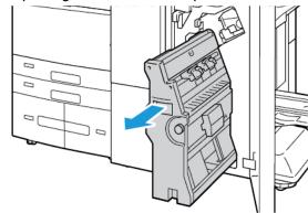
3. To remove a staple cartridge from the booklet maker, push down on the staple cartridge handle, as shown, then pull the cartridge out and up.
