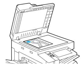
• For multiple, single, or 2-sided pages, use the duplex automatic document feeder. Remove all staples and paper clips from the pages. Insert the original documents face up in the duplex automatic document feeder, with the top of the page entering the feeder first. Adjust the paper guides so that they fit against the original documents.
