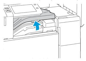
2. Pull out the hole-punch waste container.
