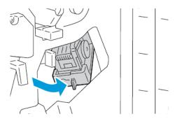
3. To remove the staple cartridge, grasp the orange handle, then pull it firmly toward you.
