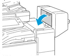
2. If the staple cartridges are not visible, grip the vertical panels at the left and right of the opening and slide the panels to the center.
