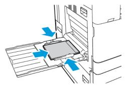
• For envelopes with a non-adhesive flap on a short edge, load envelopes face down with the flaps open, and flaps toward the left.
