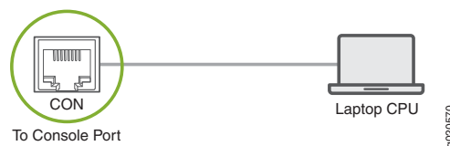
Figure 19: Connect an ACX710 Router Directly to a Management Console
