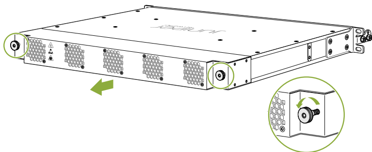
Figure 23: Remove a Fan Tray from an ACX710 Router
