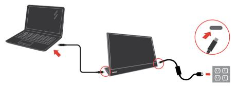
2) Connect Type-C power adapter to the left or right side of M14t and connect M14t to the mobile phone with a USB-C cable.
