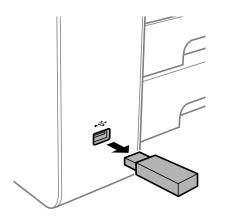
*Important:* If you remove the external USB device while operating the printer, the data on the external USB device may be lost.
