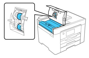
**Caution:** Using a dry cloth may damage the surface of the rollers. Do not use the ADF until the rollers are dry.
