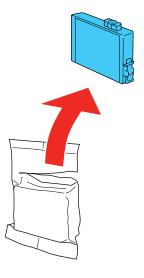
**Caution:** Do not shake the cartridges after opening the packages, or ink may leak.
