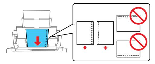
**Note:** Do not select automatic 2-sided printing for this type of paper and do not print over the holes. Select **Letterhead** or **Preprinted** as the paper type setting.
