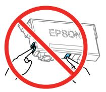
**Caution:** Do not touch the green chip on the cartridge. Install the new cartridge immediately after removing the old one; if you do not, the print head may dry out and be unable to print.
