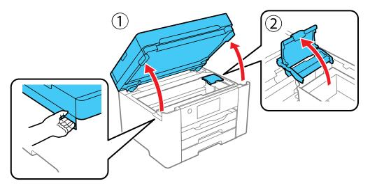
**Caution:** Do not move the print head by hand or use any kind of tool to remove a cartridge; otherwise, you may damage your product. Do not touch the flat white cable inside the printer.
