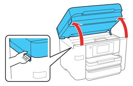
The ink cartridge holder moves to the replacement position. If the ink cartridge holder returns to the home position (far right), repeat steps 1 and 2.
