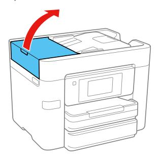
9. Use a soft, moist cloth to clean the rollers and the interior of the ADF.
