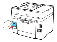
7. Press the tab on the maintenance box cover and reattach it.
