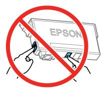
**Caution:** Do not touch the green chip on the cartridge. Install the new cartridge immediately after removing the old one; if you do not, the print head may dry out and be unable to print.
