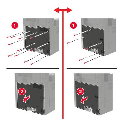
**6** Remove the controller board shield.
