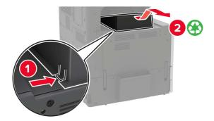
**5** Remove the adhesive cover, and then remove the paper bail.
