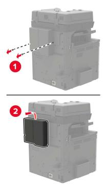
**5** Remove the controller board access cover.
