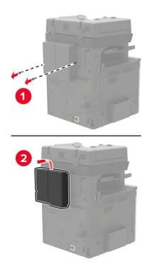
**5** Remove the controller board access cover.
