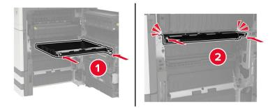
**9** Using the printhead wiper, clean the printhead lens.
