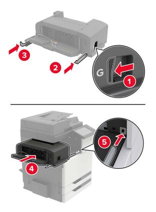
**10** Secure the finisher to the printer.
