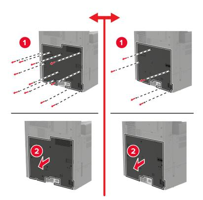
**6** Remove the controller board shield.
