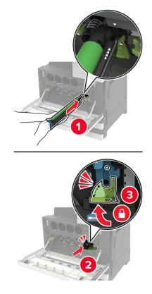
**6** Using the printhead wiper, clean the printhead lens.
