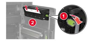
3 Open the standard trays, and then remove the jammed paper.Note: Make sure that all paper fragments are removed.
