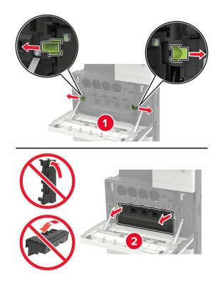
**3** Remove the photoconductor unit.
