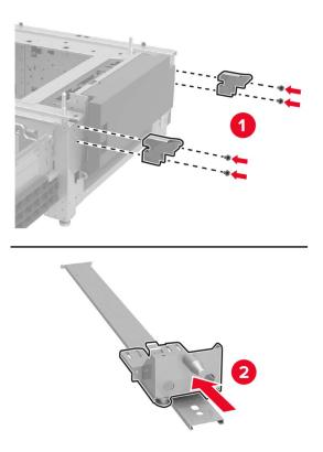
**13** Attach the rail, and then attach the mounting bracket and rail covers.
