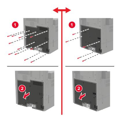
**6** Remove the controller board shield.
