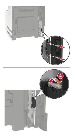
**9** Connect the wireless print server to the controller board.
