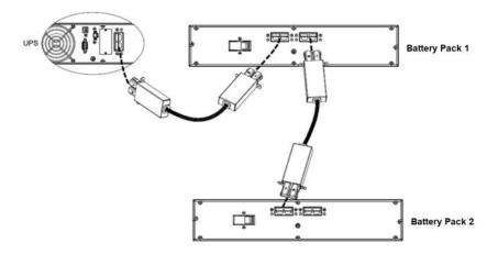
5. Stabilize the connectors to the unit and the battery pack(s) using screws. An example is shown below:
