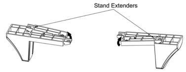
4. Stabilize the stand extenders by screwing M4 screws from the hooks to the tower stand pieces.
