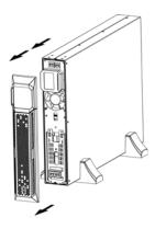
3. Turn the LCD panel such that the buttons are below the LCD screen.
