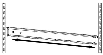
Screw a M6 screw into each of the bottom holes to fix the rail slider in place for both ends of the rail, and for both rail sliders (a total of 4 M6 screws are used here).
