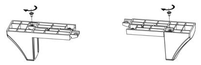
5. Orient the extended tower stand pieces as shown in the diagram below. Level and connect the hooks.
