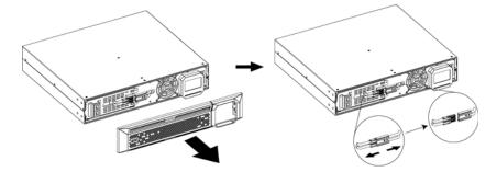
Remove the cover of the External Battery Connection Port using a screwdriver.
