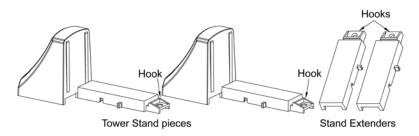
3. Orient the stand extenders as shown in the diagram below. Level and connect the extenders to the bottom of the tower stand pieces as indicated by the arrow. Make sure the hooks are properly hooked into the tower stand pieces.
