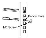
5. Insert the M6 nuts onto the support columns as show below:
