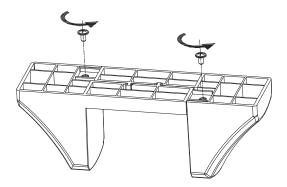
2. Bend the tower stand as shown in the diagram below:
