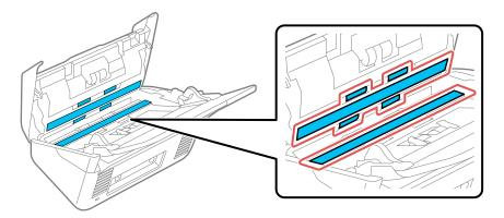
5. Use a cotton swab to wipe off any dust or dirt on the sensors.
