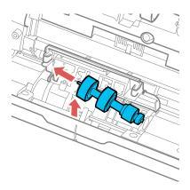
11. To install a new separation roller, insert the end of the roller into the hole on the right side and lower the other end of the roller into place.
