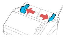
3. Load plastic or laminated cards printed side down and long edge first into the input tray horizontally, and slide them in until they meet resistance.
