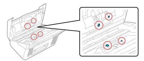
6. Wipe off any dust or dirt on the separation roller using a genuine Epson cleaning kit or a soft, moist cloth.
