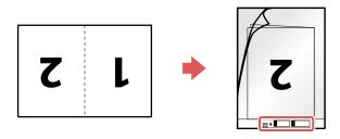
• For a photo or an irregularly shaped original, load it in the center of an optional carrier sheet with the printed side face down. Make sure the illustration on the front edge of the carrier sheet is facing up.
