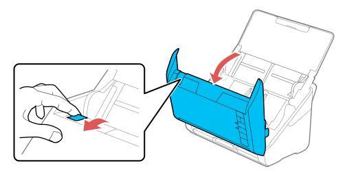
5. Press down on the pickup roller cover latch and pull up the cover to remove it.
