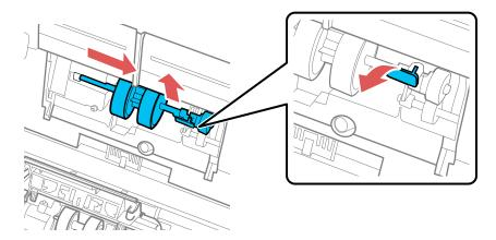
Note: Do not use force to pull out the pickup roller; doing so may damage the inside of the scanner.
