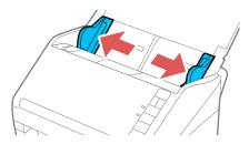
4. Load envelopes vertically in the input tray with the printable side down and the flap facing as shown. Slide in the envelopes until they meet resistance.
