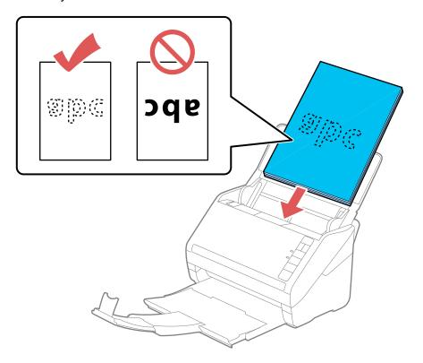
• If you are loading paper business cards, load up to 15 (DS-530 II/DS-575W II) or 30 (DS-770 II) cards printed side down and long edge first into the input tray horizontally, and slide them in until they meet resistance.
