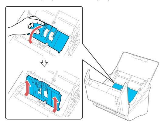
6. Pull down the tab on the pickup roller and slide the roller to the right to remove it.
