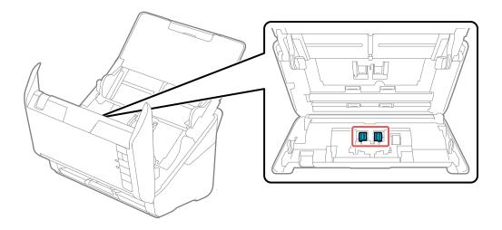
7. Wipe off any dust or dirt on the pickup roller using a genuine Epson cleaning kit or a soft, moist cloth.
