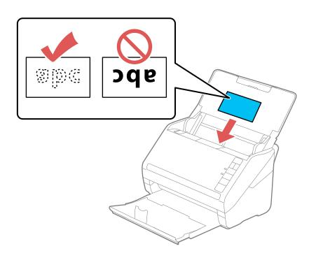
• If you are loading hole-punched originals, load them with the holes facing down or to the side as shown. The holes must be within 1.2 inches (30 mm) of the edge of the originals.
