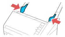
**Note:** If you are scanning originals that are 15.5 inches (393.8 mm) or longer, support the original as it enters into and ejects from the scanner as shown.
