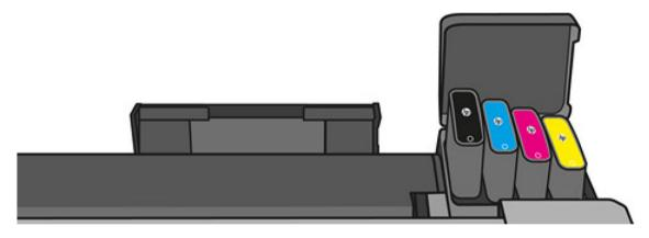
4. Insert the new ink cartridge. Make sure that you insert the ink cartridge into the slot that has the same colored letter as the cartridge you are installing.
