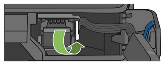
12. Insert the tubes connector into the printhead.
