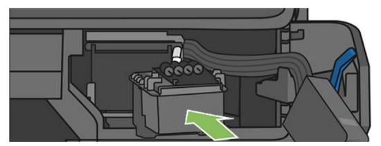
Check that you have correctly latched the printhead (white latch), see Replace the printhead on page 101.
