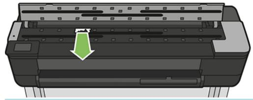
**CAUTION:** Do not move the paper sideways as it could damage the scanner.
