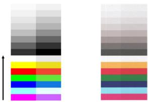
Sometimes the color mismatch between adjacent modules can be enormous, showing a serious scanner malfunction, as in the following example. If this occurs, see Completely wrong colors on page 162.
