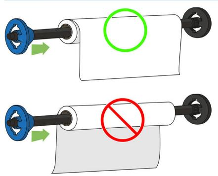
Ensure both ends of the roll are as close to the spindle stops as possible.
