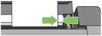
Feed the paper into the printer. Feed the paper into the printer until you feel resistance and the paper bends slightly. When the printer detects the paper, it beeps, and feeds in the paper automatically
