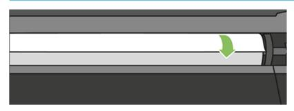
6. Roll the paper into the printer until you feel resistance and the paper flexes slightly. When the printer detects the paper, it beeps, and feeds in the paper automatically.
