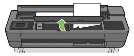
Remove the sheet from the printer.
