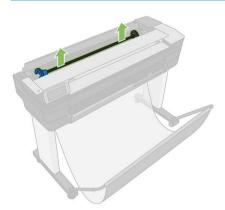
3. The spindle has a stop at each end to keep the roll in position. The blue stop can be removed to mount a new roll; it slides along the spindle to hold rolls of different widths. Remove the blue paper stop from the end of the spindle.
