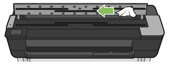
5. For more thorough cleaning, clean the calibration surfaces and the feed rollers.
