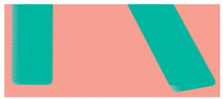
If edges of objects or lines appear to be poorly defined or lighter in density, and you have already set the printquality slider to Quality in the driver dialog, select the custom print-quality options, and try setting the quality level to **Speed**. See Printing on page 41.
