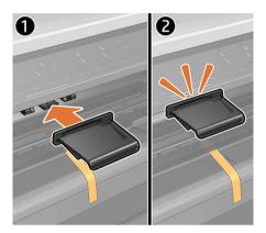
The refeed preventers are designed to prevent this situation from occurring. Make sure that they are always installed.
