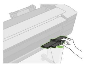
4. Load sheets of paper into the tray with the printed side facing outwards. Ensure that the sheets are all of the same size, and that they reach the bottom of the tray.
