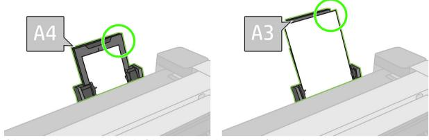
If the paper is hanging over the back of the input tray as shown, it may fail to load.
