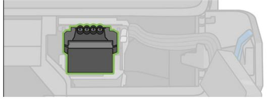
9. Remove the printhead. Handle it with care to avoid getting ink on the connections.
