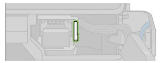
8. Raise the lever to release the printhead.
