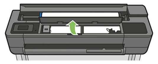
3. Remove any of the jammed paper that you can lift up and out from the top of the printer.
