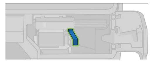
6. Raise the blue lever to release the tube connector and store the tubes connector on the tubes connector holder in the printer door.
