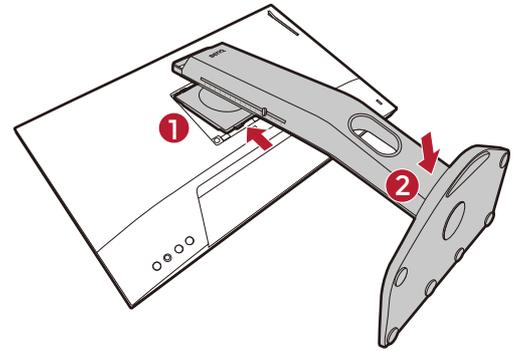
Carefully lift the monitor, turn it over and place it upright on its stand on a flat even surface.
