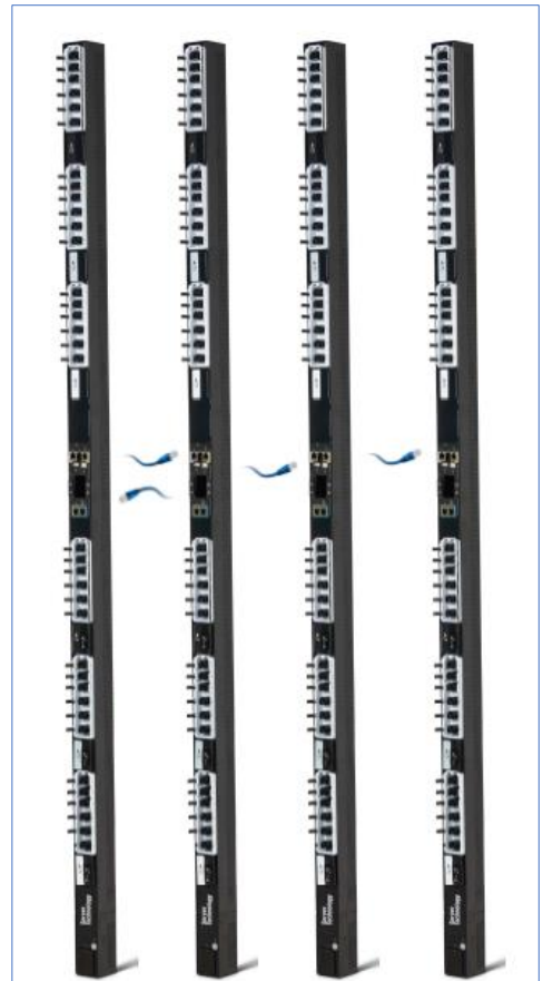
PRO3X PDU Linking: One master unit with up to seven link units. Two cables needed between the master and the first link unit – one for linking and the other for redundant back feed power.
