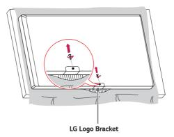
2 After removing the screw, remove the LG Logo Bracket. When re-attaching the LG Logo Bracket, repeat the process in reverse order.
