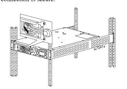
NOTE: Pull the strap provided on the connectors for disconnecting the battery. Do not pull the wires.
