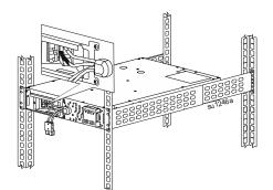
Connect the red color internal battery connector to the red color receptacle in the battery module. Be sure that the connection is secure.
