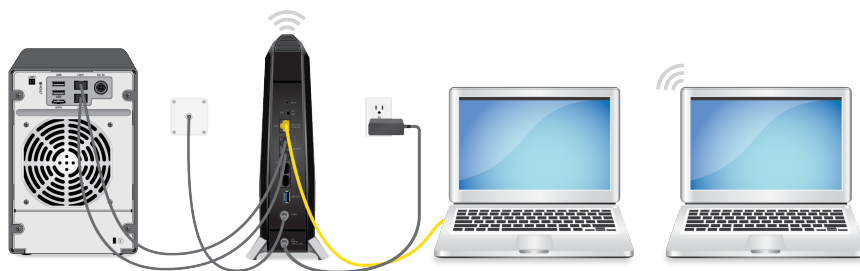
Figure 5. Ethernet port aggregation
